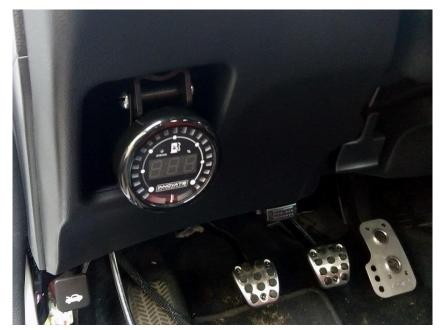
• To mount the gauge in this location, simply cut a 1" hole at the back of the pocket to fit the wiring through, using a drill bit or hole saw. Then use double sided tape to mount the gauge pod.
