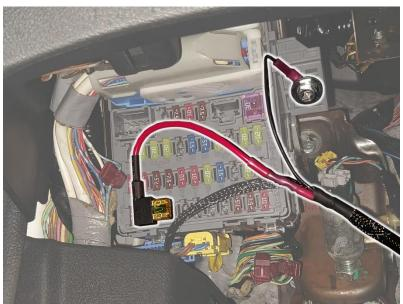
18. Fasten the Ring Terminal End of the SiriMoto Chassis Harness to ground. A good option is to use the 10mm Hex Head Bolt found to the right of the fuse box. To do this simply remove the bolt, slide the ring terminal in place and tighten the 10mm bolt.
